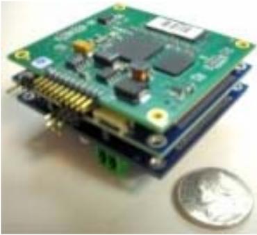
Figure 3. The one-ounce Embeddable Programmable Instrumentation Circuit (EPIC).
