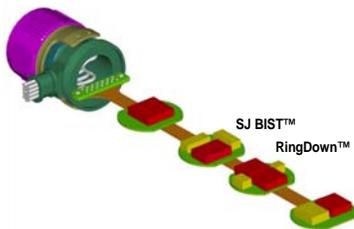
Figure 2. Circuitry added to the back shell of a wiring
