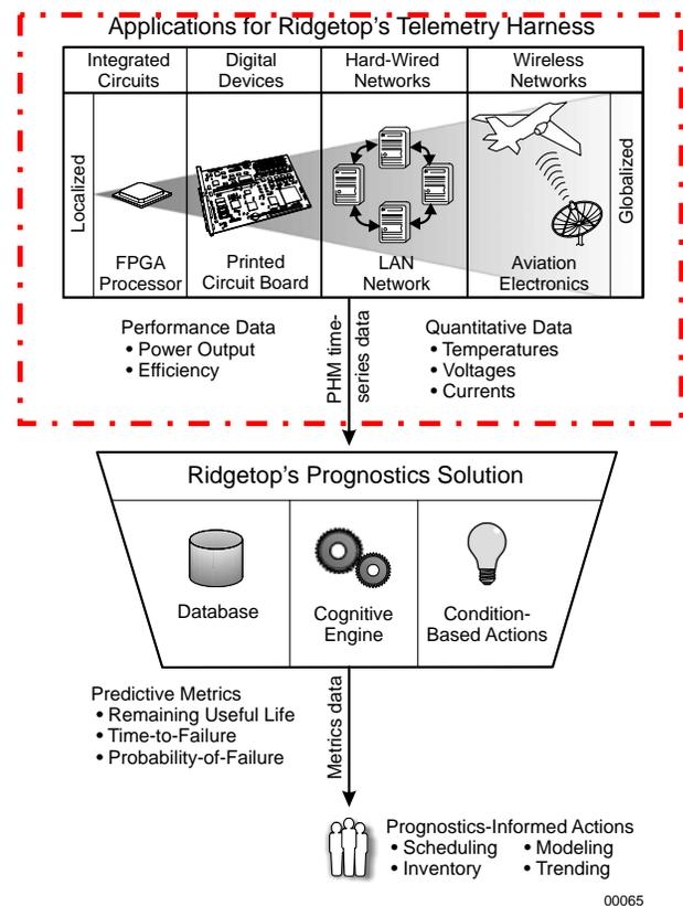
Figure 4. Application, scalability, and process flow of Ridgetop's telemetry harness and Sentinel Network™.
