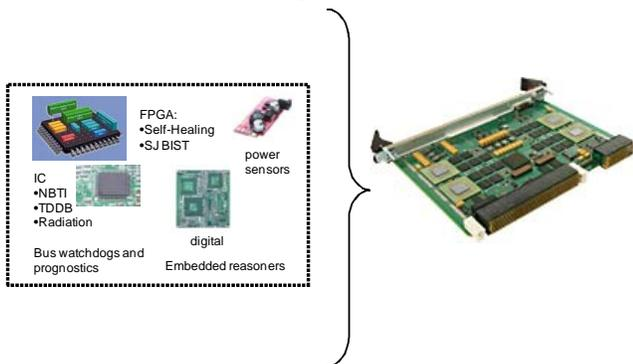
Figure 1. Printed circuit boards (PCBs) or modules can be “prognostic-enabled” by using sensors that employ physics-of-failure methods.
